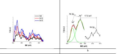
Figure 4.4 a) Ni 2p depth spectra acquired after surface etching with Ar ions; b) Deconvolution of the signal of the N15 thin film, showing the new components
