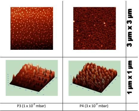
Figure 3.4 The influence of the oxygen pressure on the morphology of the AZO films; the change of the way in which the surface is organized takes place at an intermediary pressure, between the values used for depositing the two samples shown above
