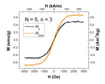
Figure 4.10 Hysteresis curves traced for the field parallel and perpendicular to the film surface, for the samples with N = 5
