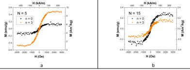
Figure 4.9 The effect of adding Al (*n* pulses per sequence) to the composition of ZnO:Ni on the hysteresis cycles
