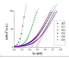
The increase of  $E_g$  could be caused by the stress in the film In our case the stress is of intrinsic origin, being caused by the structural defects in the material. In order to compute the stress values for the samples C1-C3, for which we only have the (002) maximum in the diffraction patterns, we used the following formula [41] for the stress in the plane parallel to the film surface:
