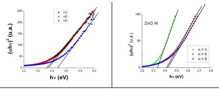
Figure 4.14 The increase of the band gap with the number of pulses of Al for ZnO:(Ni, Al). In the image on the right are shown, for comparison, the BG of the AZO samples deposited with identical values of n per sequence
