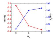
Figure 3.13 The change of the stress and band gap values with changing Al concentration (samples C1 - C3)
