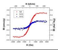
Figure 4.8 The M-H curves for the TF of ZnO:(Ni, Al), recorded at 300 K in the H<sub>11</sub> configuration
